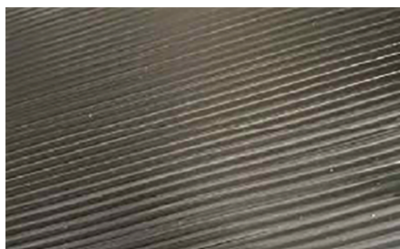
Embossed slip resistant walking surface X4 magnification
